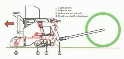
Top quality strong cutting knife (schematic drawing nr.1) (img. cutting knife).
