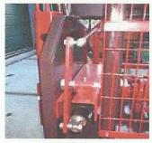
Middle disc coulter for splitted rolls (img. middle disc coulter)
