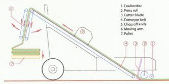
The cutter head of the Big Slab is the same as in the big tick (schematic drawing nr. 1,2 and 3). Strong cutting blade and sharp edges due to the coulter discs. The soil is leveled by the heavy frame weight and solid press roll. A middle disc coulter can split the slab in two parts. The thickness of the sod is adjusted with the automatic thickness control (img. Big Slab automatic thickness control).
