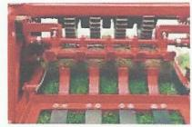
Cross-conveyor, hydraulic driven, with speed adjustment for ease of stacking. Conveyor belt is smooth so that it does not damage the turf (img. roll on crossconveyor). The belt it is special material, almost unwearable The special pallet carrier can be hooked on and off like regular agricultural equipment (optional).
